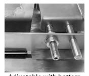
Adjustable with bottom gage for precision cuts
